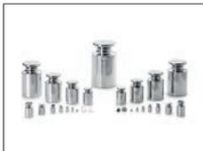
OIML / ASTM Weights (with calibration certificate)
